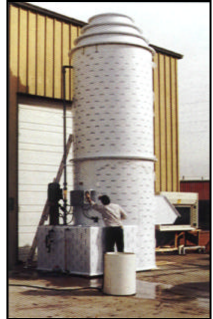
15,000 ACFM Dakota Scrubber™ during quality control inspection at Dakota International, Inc.'s fabrication facility
